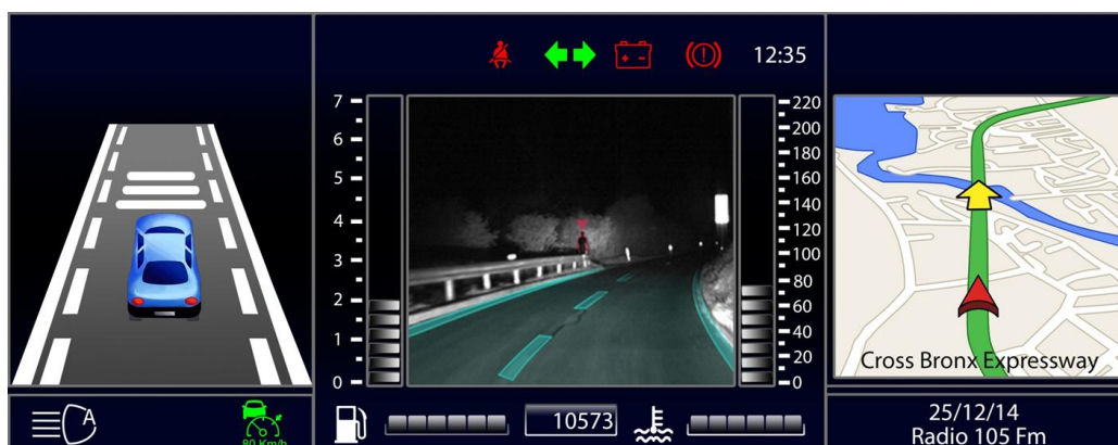
Figure 3. The HMI design for the DESERVE ADAS functions
