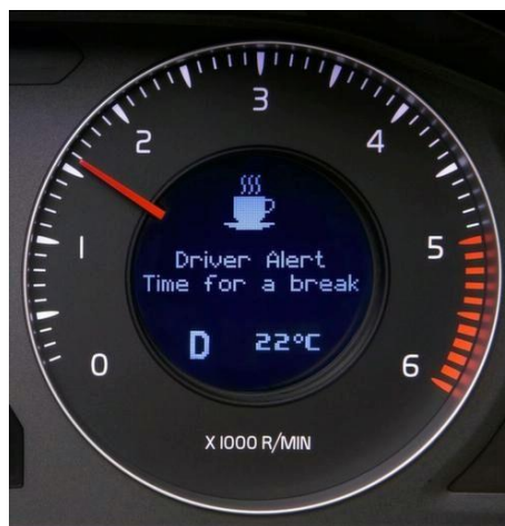
Figure 11 - Volvo Driver Alert Control warning message in the dashboard display
