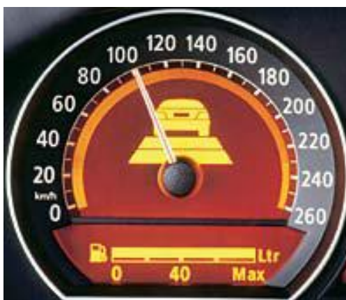
Figure 8 – ACC light in the speedometer when approaching a slower car
