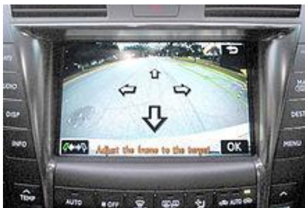
Figure 6 - Lexus backup camera system showing the parallel park setup screen
