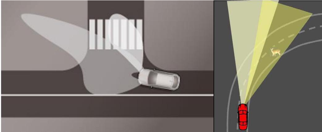
**Figure 4. Example of the Adaptive Light Control**
