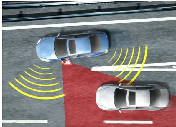
**Figure 3. Blind-spot assistant ultrasonic sensors for safe lane changes**
